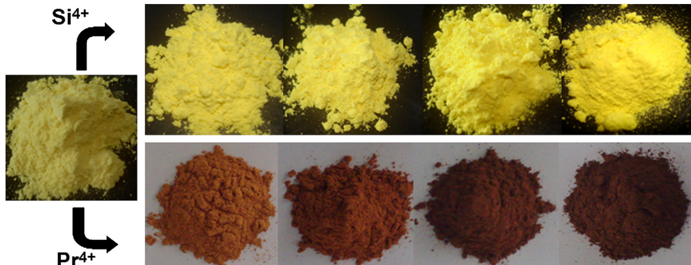
Fig. 4. Photographs of Y_{6-x}Si_xMoO_{12+\delta} and Y_{6-x}Pr_xMoO_{12+\delta} pigments.
